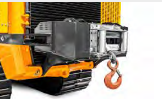
Recovery (Towing) rear winch 6 ton capacity
