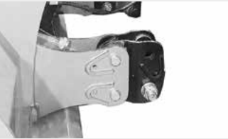
Extended 3 point linkage
