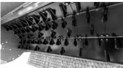
Interchangeable bolted on spike counter blade can adjust final product size while operating
