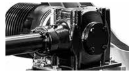
Reversible gear box for frontal attachment (optional)
