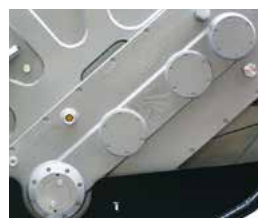
Dual transmission with side gearbox increase power delivery to the rotor
