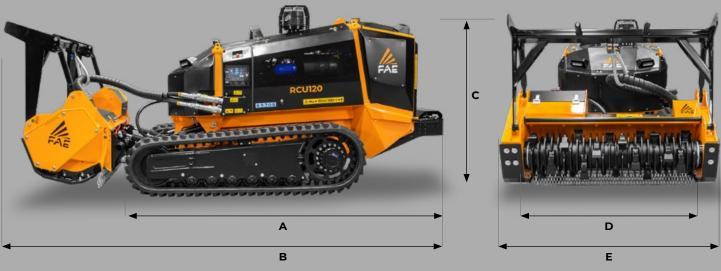
A Overall lenght without attachment124B Transport lenght with BL4/RCU120 attachment on ground171
