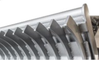
Rear hood grill allows larger material to be held back and crushed again for optimum results
