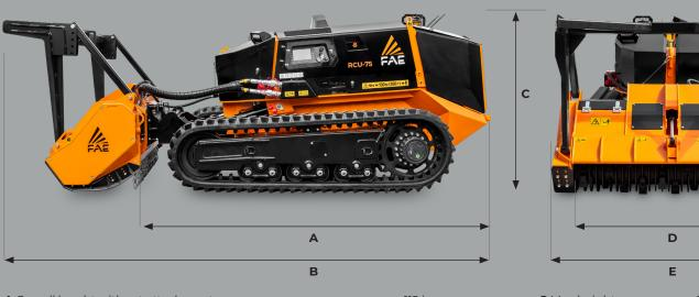
A Overall lenght without attachment **B** Transport lenght with BL2/RCU attachment on ground 112 in 160 in **C** Max height 61 in **D** Overall track width 67 - 83 in **E** See attachements table
