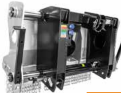
Hydraulic side shifting allows the stump cutter to move easily, quickly, and accurately while working close to plants and crops without damaging them
