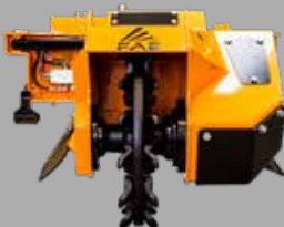
Stump cutter for the RCU75 remote controlled tracked carrier
