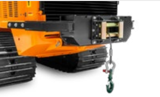
Rear winch with 6 t pulling power
