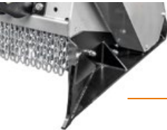
Penetration skids help the machine to better penetrate the soil
