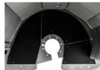
**Interchangeable Hardox® internal and side guards**
