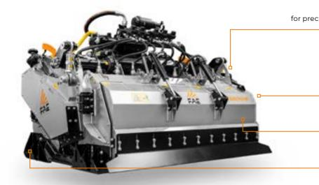
Variable geometry chamber for precise earthworking and to obtain an optimized mixture
