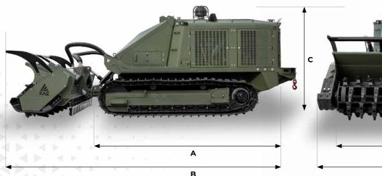
A Overall length without demining head 4950 mm **B** Transport lenght with 300/TD attachment on groundand winch 6500 mm
