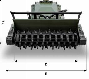
C Max height 2700 mm D Overall tracks width 2360 mm (660 pads) E See attachements table
