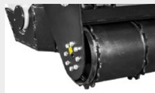
Hydraulic controlled roller helps with compaction and working uneven terrain
