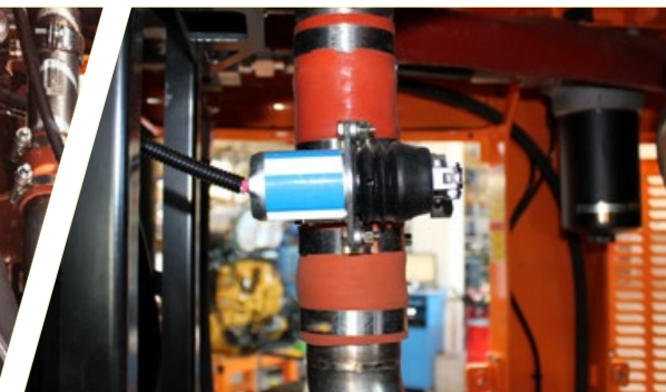
Air shut-off system
