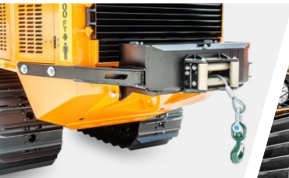
Rear winch - rated towing capacity: 6t
