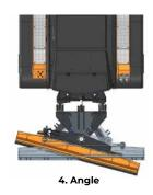
The 8-way movement allows you to tilt (1), lift (2), roll (3) and angle (4) the blade, all from the cab or remote control of your PT-300 D:MINE!
