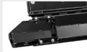
**Dozing blade** to level the crushed material
