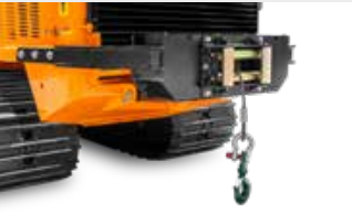
Rear winch with 6 t pulling power
