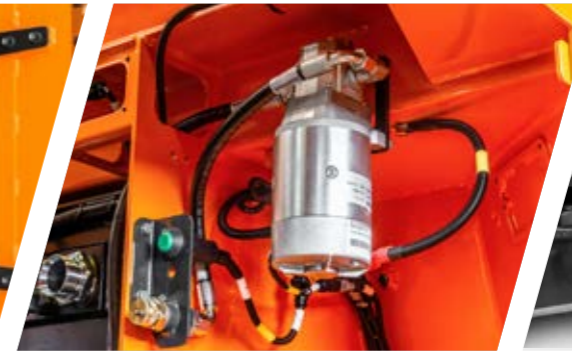
Oil top-off pump (service package)
