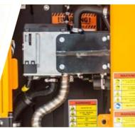
Pre-heating system for engine and hydraulic oil
