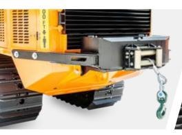
Rear winch - rated towing capacity: 6t
