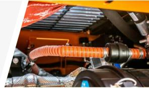
Ejector (heavy duty filtration package)
