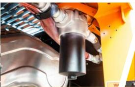
Drainage filter (heavy duty filtration package)
